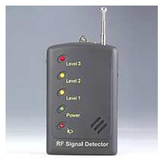
The **SIS-055SRV** can detect the popular microtransmitter, wireless CCTV camera, wireless phone, wireless microphone, wireless tap and cellphone from 50 MHz ~ 6.0 GHz.
